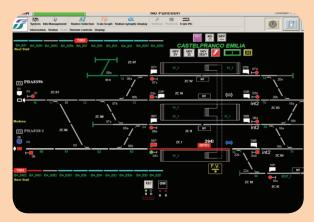
The use of train information provided by ETCS Levels 2 and 3 allows to perform and/or improve various useful functionalities like "consistency check" between planning and real situation (verification of "Train Running Number ID", Train category, train length/convoy type, train characteristics), to trace conditional route/itinerary and thereby to anticipate and manage potential conflicts in a faster and efficient way.
