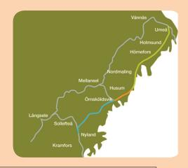
The Ådal Line carries both passenger and cargo traffic. It includes over 35 level crossings and runs between Sundsvall and Västeraspby. The line is 180 km long. 50 km are new (Härnösand – Mörtsal). ERTMS Level 2 has been chosen for the implementation and when the line has been completed, the capacity will increase from 8 - 10 trains perday to 50 - 60 trains per day.
